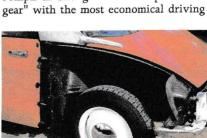
To change a rear wheel, undo one bolt, lift off the mudguard and hey presto! Note two pegs at leading edge of rear guard
